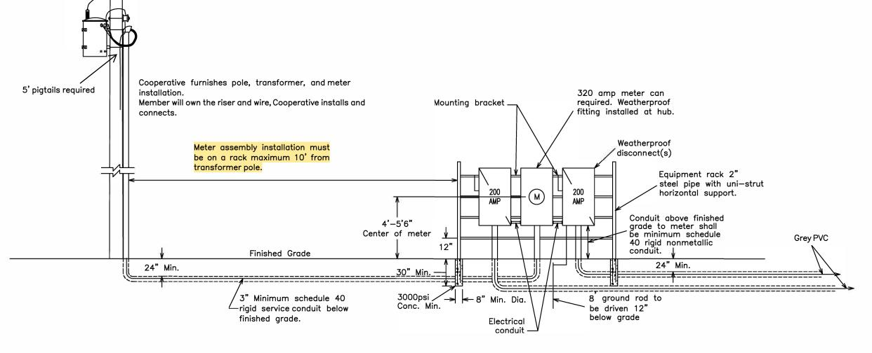
FOR THE MEMBER'S SAFETY, WIRING INSTALLATIONS SHALL CONFORM TO THE REQUIREMENTS OF THE NEC AND NESC.
